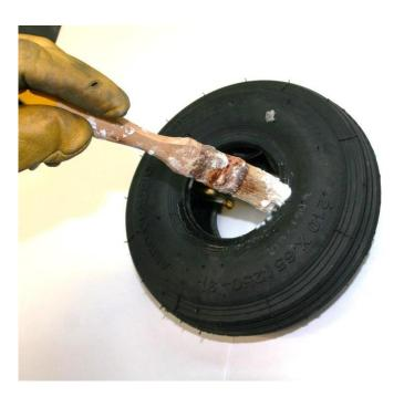
Push the first tire bead, the lower one, of the tire and tube assembly onto the wheel hub. The valve has to point upwards.
