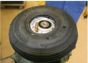
Grease the upper tire bead with tire bead lubricant and push the tire bead onto the wheel hub.
