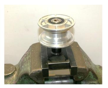
Insert the tube into the tire. To simplify the tire mounting we recommend to heat the tire in an oven (150°C, 10 minutes), that improves the smothness of the tire. After heating, insert the tube. Protective hand gloves are highly recommended.
