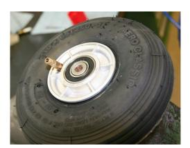
Inflate the tire with pressurized air (4,0 bar / 58 PSI rated pressure) in a proper safety cage and sufficent safety distance. If no safety cage is available pay maximum attantion during inflation and adhere a maximum safety distance. The use of a valve extension is highly recommended. After diffusion and leakage test mount the valve cap.
