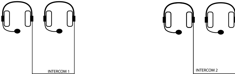
Figure 7.2.: The intercom function is active and the isolation function is active as well. All participants on INTERCOM 1 and INTERCOM 2 can talk to each other, however, the two groups INTERCOM 1 and INTERCOM 2 are isolated from each other.
