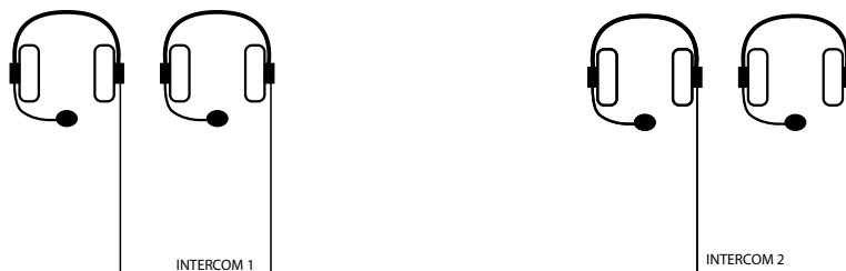
Figure 7.3.: The intercom function is not active. No participant can talk to any other participant.
