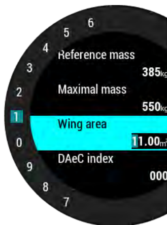
Grey rectangle indicates the character which is being edited. Edit character with rotary switch.
