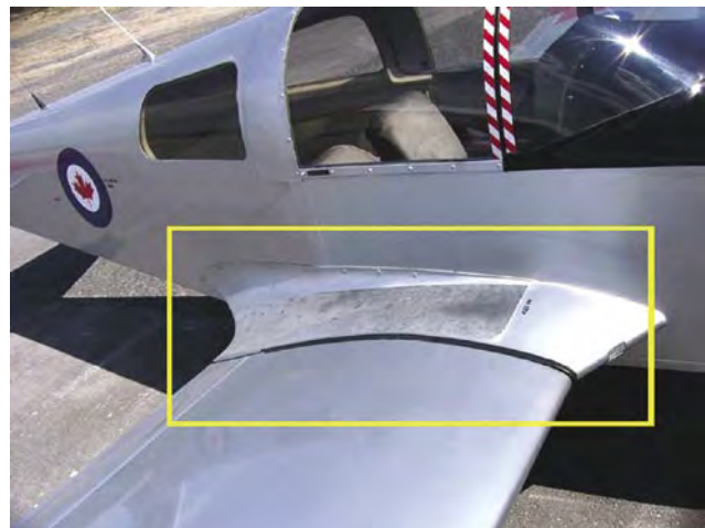
Figure 4-6. A wing root can cause interference drag.
