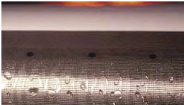
Figure 6-48. TKS weeping wing anti-ice/deicing system.
