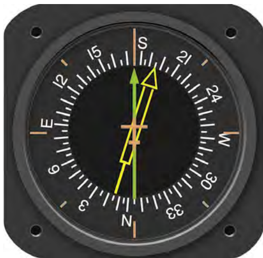
Figure 7-30. Driven by signals from a flux valve, the compass card in this RMI indicates the heading of the aircraft opposite the upper center index mark. The green pointer is driven by the ADF.
