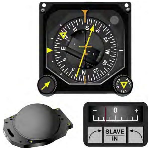
Figure 7-29. Pictorial navigation indicator (HSI, top), slaving meter (lower right), and slaving control compensator unit (lower left).
