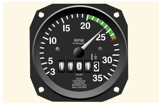
Figure 6-8. Engine rpm is indicated on the tachometer.
