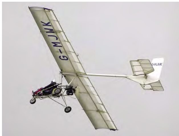
Figure 1-20. A typical ultralight vehicle, which weighs less than 254 pounds.
