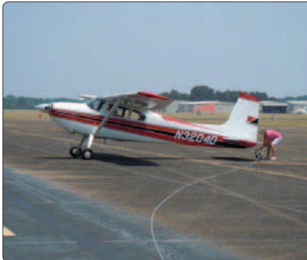
Figure 12-6. It is both the tow pilot and glider pilots responsibility to check the condition of the tow rope before flight.
