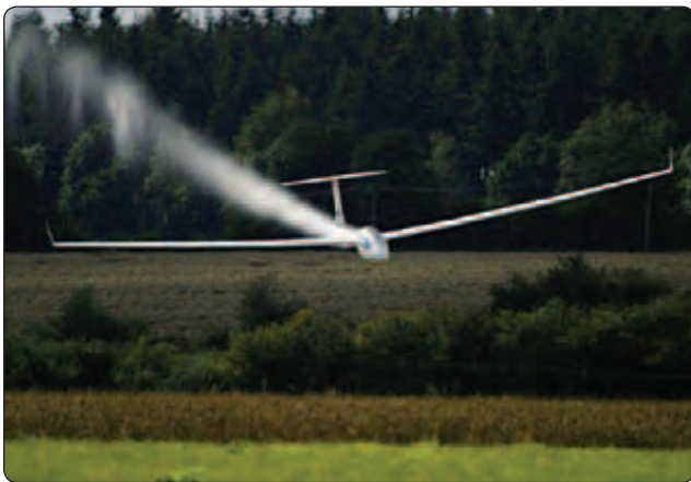
Figure 2-4. Sailplane dropping water ballast before landing.
