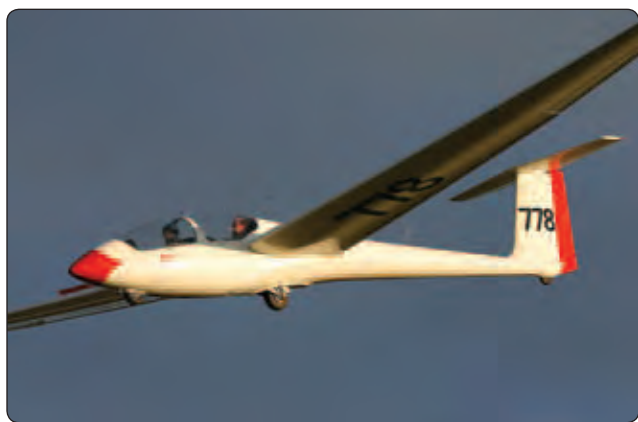
Figure 1-6. A sailplane is a glider designed to fly efficiently and gain altitude solely from natural forces, such as thermals and ridge waves.
