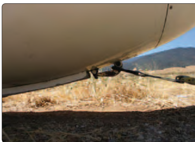
Figure 6-11. Schweizer-type tow hook.
