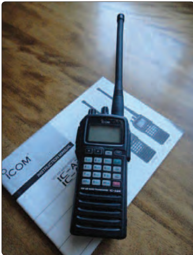
Figure 12-16. On a cross-country tow, the tow pilot and glider pilot should have two way communication using portable radios.
