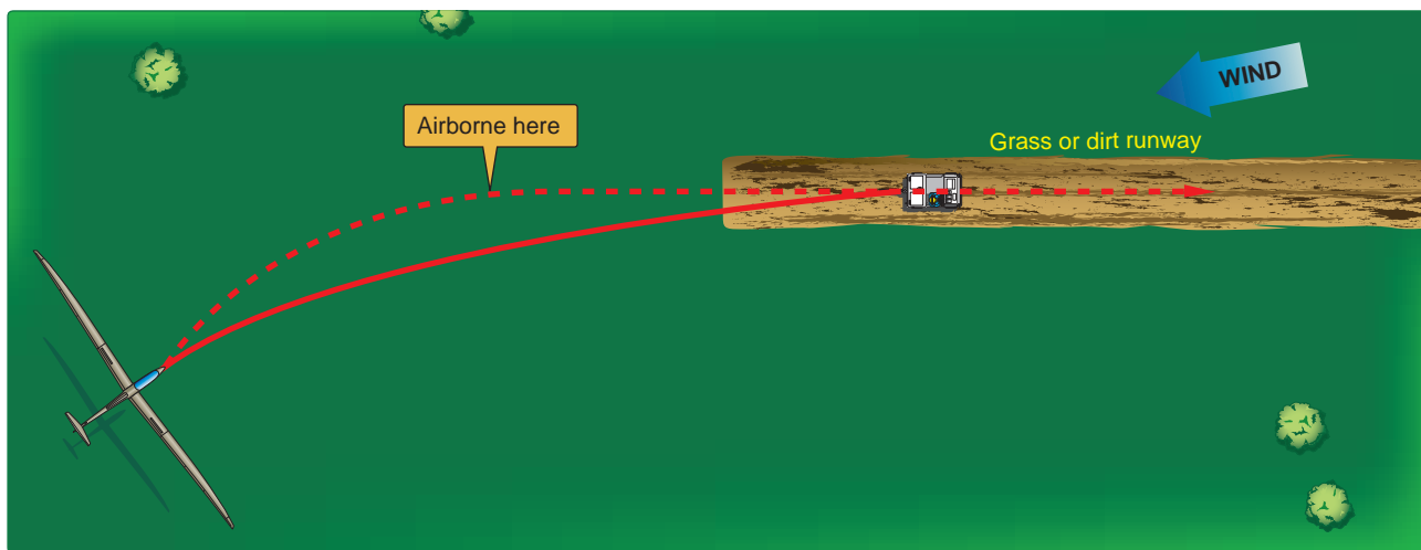
Figure 7-17. Ground launch procedures.
