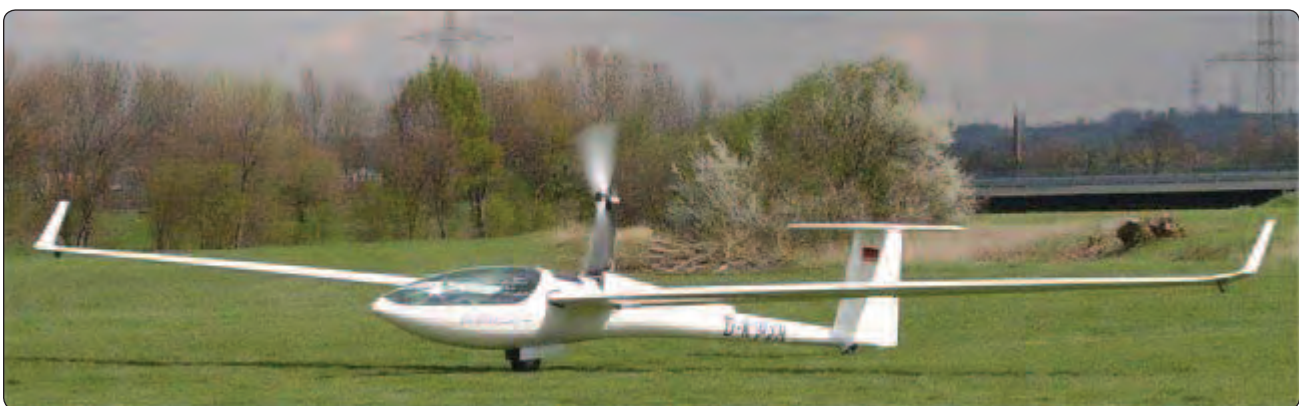
Figure 2-16. A DG-808B 18-meter high-performance glider in self-launch.
