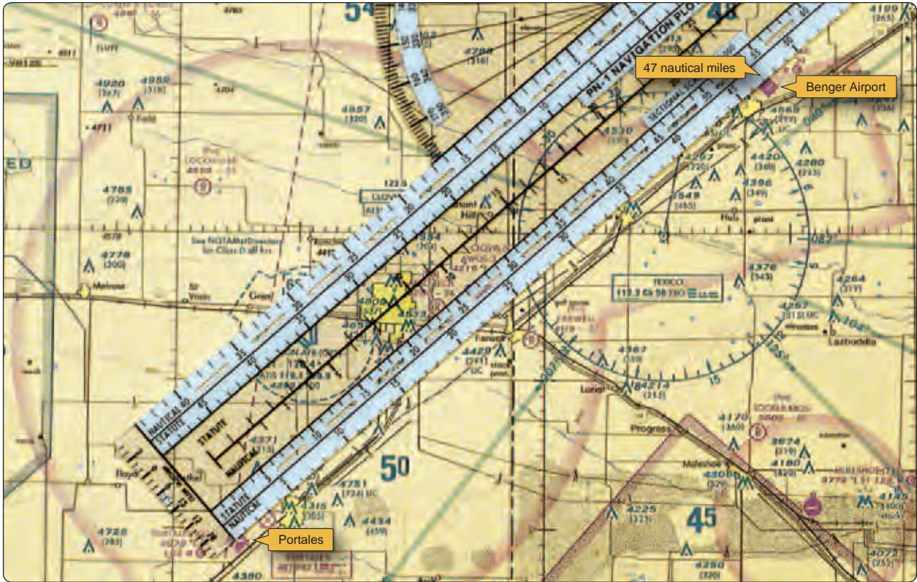
Figure 11-5. Measuring distance using the navigation plotter.
