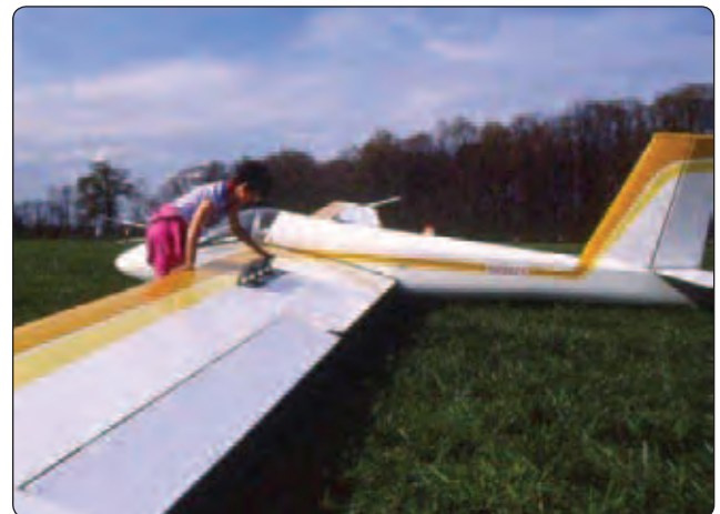
Figure 6-14. Positive control check of spoilers.
