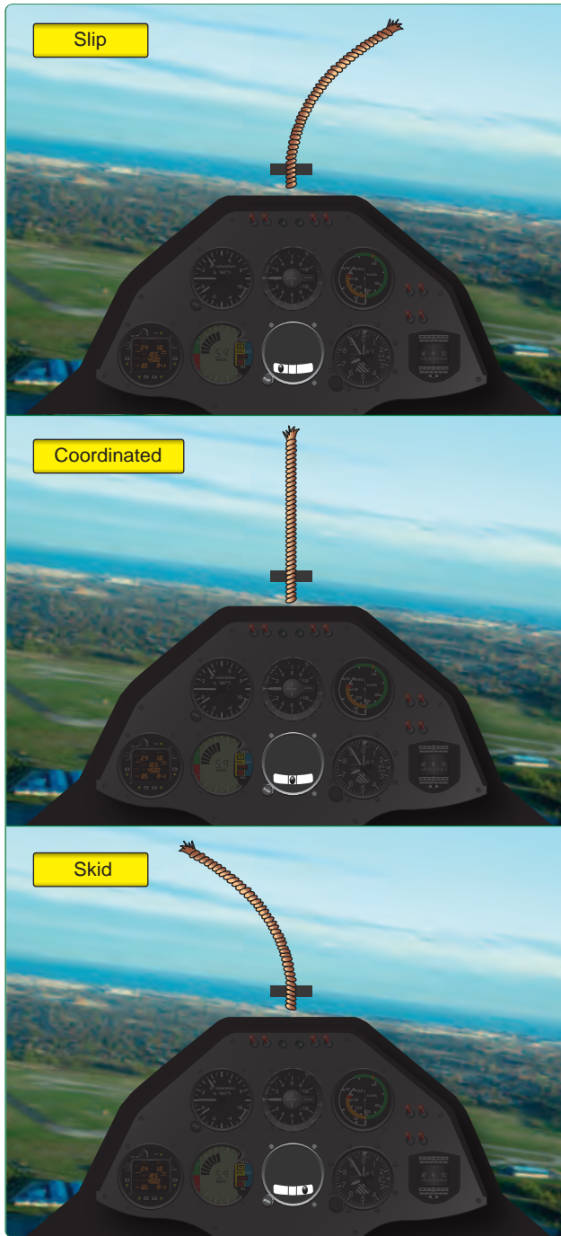
Figure 4-30. Left turn condition indications of a yaw string and inclinometer.
