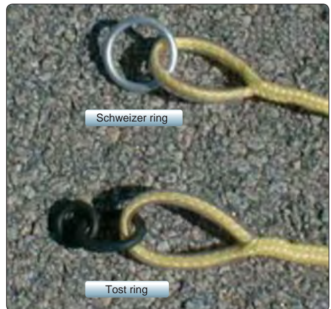
Figure 8-10. Examples of Schweizer and Tost tow rings.
