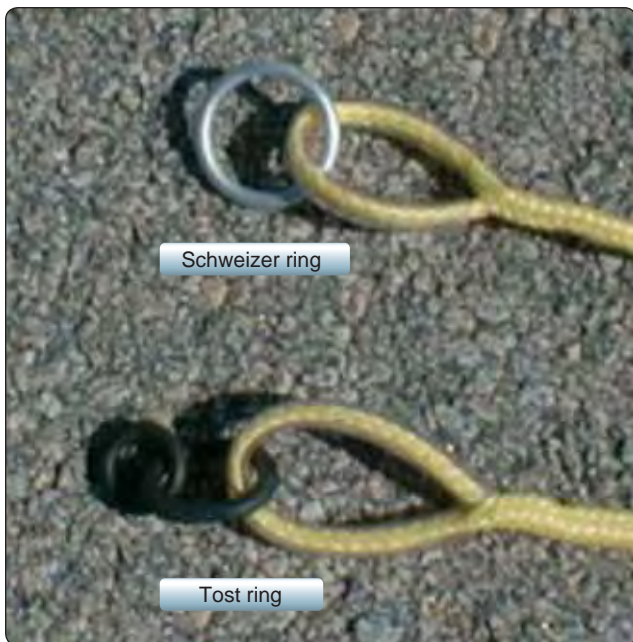
Figure 12-5. Schweizer tow ring and a Tost tow ring.
