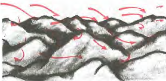
FIGURE 170. Windflow over various types of terrain. The many deviations from these patterns depend on wind speed, slope profile, and terrain roughness.
