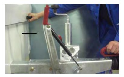
**Test:** Activate the hand brake and push the trailer back by hand.
