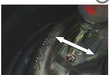
See on this picture how to move the star wheel arrow wise with a screwdriver. While adjusting, turn the wheel slowly in driving direction. Continue until the wheel blocks. Then move the star wheel back against the arrow (still turning the wheel in driving direction) until you can hear and feel that the brake lining is very, very smoothly touching the brake drum. If the lining is worn unequal, you may have to do this again several times. **Attention:** The arrow shows a different
