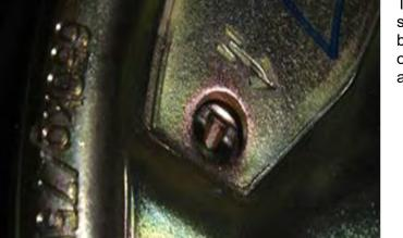
Through the second, inner hole you can see the star wheel for adjusting the brakes. The impressed arrow on the side of the hole shows the direction for adjusting. A. SPINDELBERGER Fahrzeugtechnik GmbH
