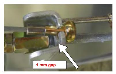
**Important:** Make sure the brake rod is properly adjusted! The gap (arrow) between the long nut and the U- shaped equalizing lever has to be **1mm** with released hand brake! Make sure, that the brake rod is not bent! Straighten if needed!
