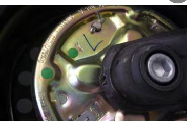
Open both the green plugs on the brake plate with a small screwdriver (rear of the brake drum). On this picture, you see the left side brake.
