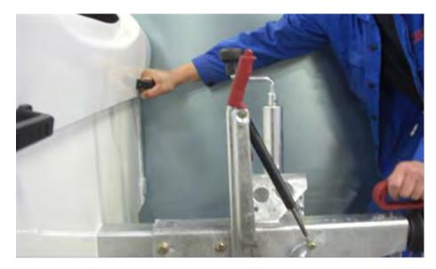
After the trailer is on its wheels again, please check the correct adjustment. Activate the hand brake and push the trailer back by hand. During you are pushing the lever has to move back from itself until it is **90°** to the tongue (not more than **90°**!).
