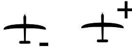
Figure 2.4.: Aircraft below (little minus-sign) and above (little plus-sign) the own ships current altitude.
